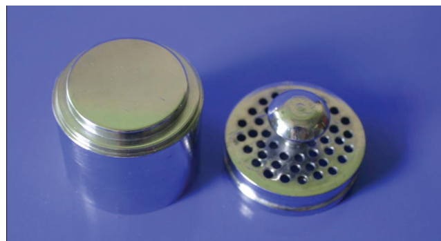
Fig. 3. Platform and tray for impression used to fabricate the specimens for the surface roughness test.
