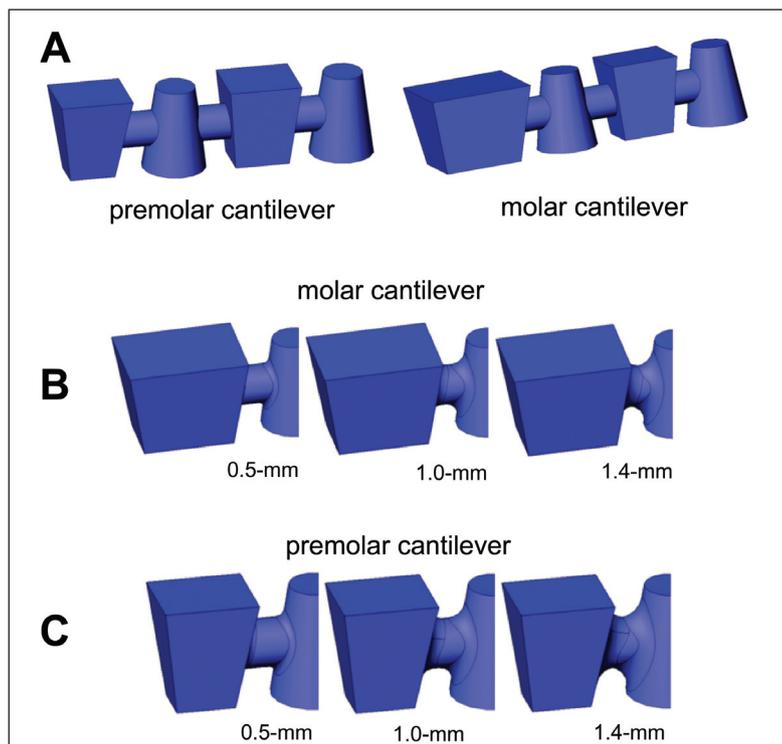
**Fig. 2.** (A) Simplified model of the titanium framework design with a premolar (left) and molar (right) cantilever. (B) 0.5-mm, 1.0-mm, and 1.4-mm fillets in the molar cantilever (from left to right). (C) 0.5-mm, 1.0-mm, and 1.4-mm fillets in the premolar cantilever (from left to right).
