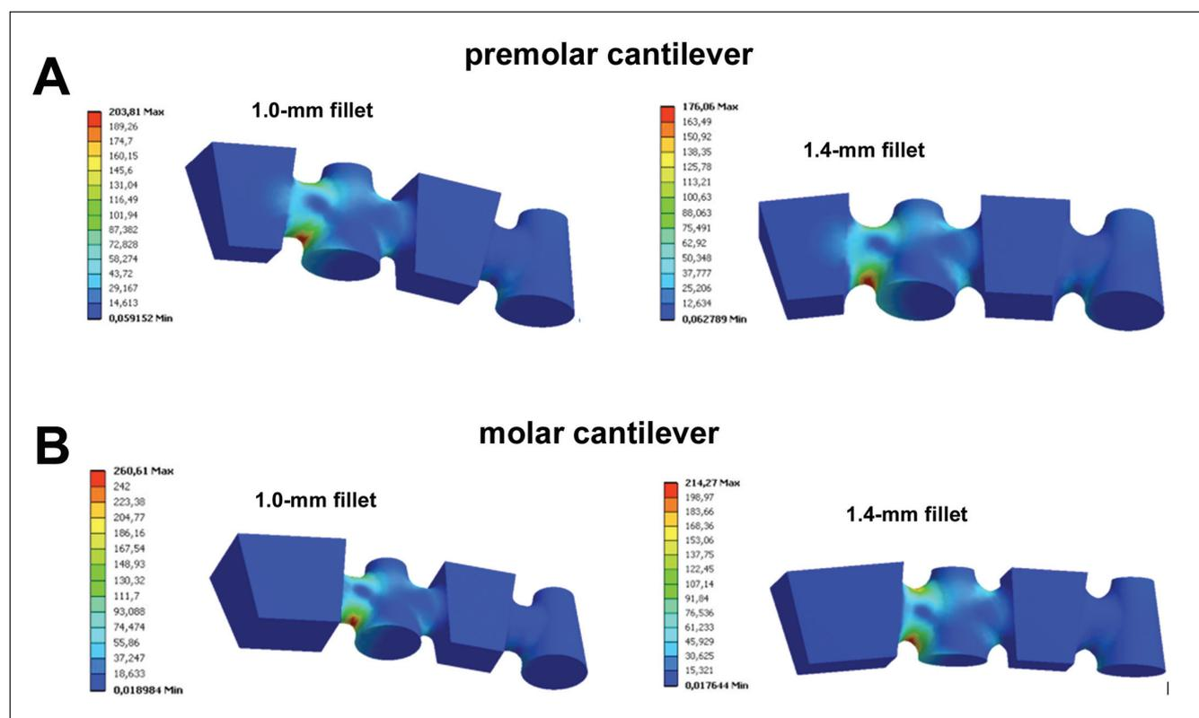
Fig. 5. Fixed dental prosthesis framework design. Connector area of 9.05 mm<sup>2</sup>. (A) Premolar cantilever; 1-mm (left) and 1.4-mm (right) fillet. (B) Molar cantilever; 1-mm (left) and 1.4-mm (right).
