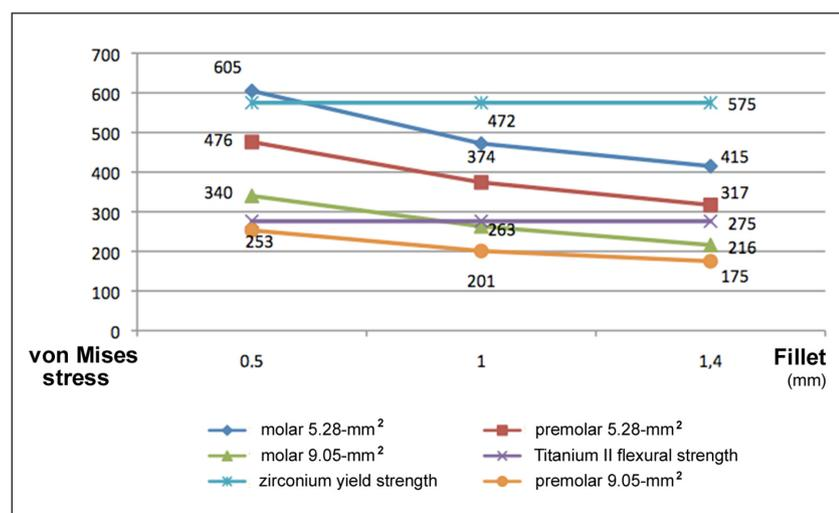
Fig. 4. Graphic representation of the von Mises stresses obtained under a 125 N load for different CAD designs.
