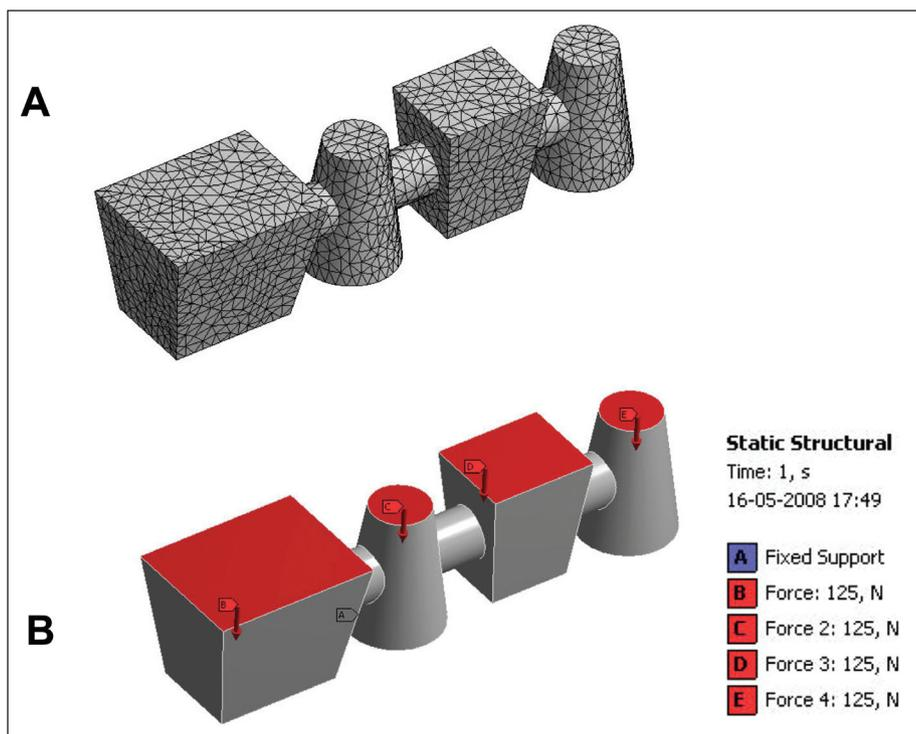
**Fig. 3.** (A) Finite element mesh of the simplified model of the cantilever-fixed dental prosthesis framework in titanium. (B) Load distribution over the fixed partial denture (500 N, 125 N per tooth).
