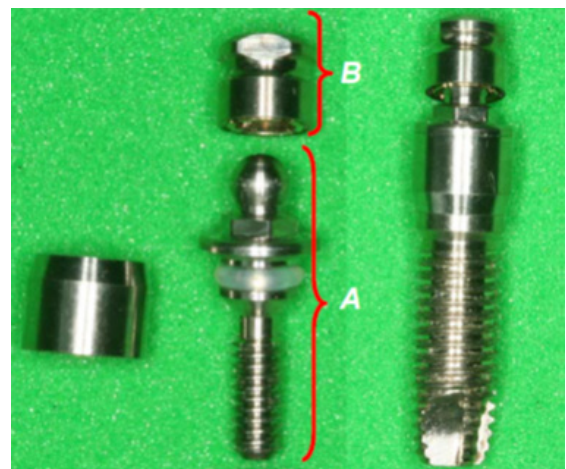
Figure 2. Ball Attachment Dal Ro ® , 4-mm height: A – male component; B – female component.
