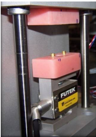
Fig. 4. Load cell Futek S shape, model Futek® LSB 300,
