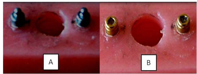
Fig. 1. (A) The Dalbo-Ball® system of 3 mm height screwed to the implants in the acrylic block; (B) The Locator® attachment system of 3 mm height (titanium alloy coated with TiN) screwed to the implants in the acrylic block.
