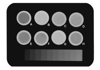
**Fig. 1.** Representative radiography of test samples near the aluminium stepwedge (bottom): a - Acroseal; b - Endofill; c - Epiphany; d - Sealapex; e - Sealer 26; f - Endomethasone; g - AH Plus; h - MBP.
