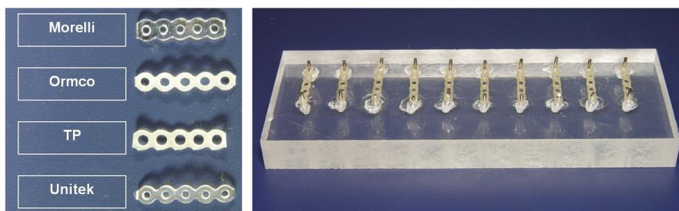
Fig. 1. Tested synthetic elastic chains and the experimental set-up.
