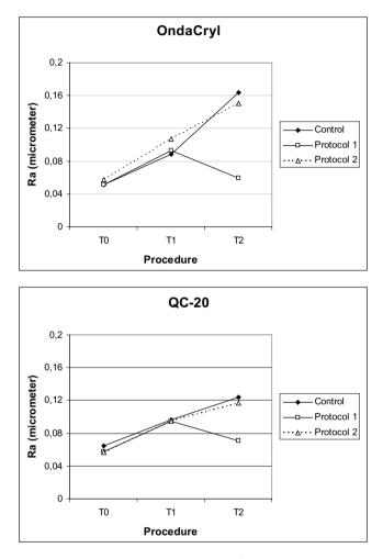
Fig.1. Ra mean values (in micrometers) of OndaCryl and QC-20 resins according to disinfection treatment groups and number of disinfection procedures. Control and Protocol 2 (345 W/6 min) groups showed similar behavior. A significant decrease of surface roughness (P<0.05) occurred after two microwave disinfection procedures with Protocol 1 (690 W/6 min).
