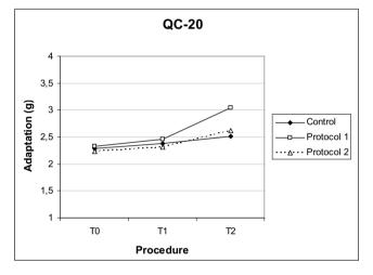
**Fig.2.** Baseplate adaptation mean values (in grams) of OndaCryl and QC-20 resins according to disinfection treatment groups and number of disinfection procedures. Control and Protocol 2 (345 W/6 min) groups showed similar behavior. Significant poorer adaptation (P<0.05) was measured after two microwave disinfection procedures with Protocol 1 (690 W/6 min).
