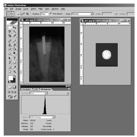
Fig. 1. Adobe Photoshop<sup>®</sup> software showing the image obtained of tubes and standard discs methods and areas of interest selected.
