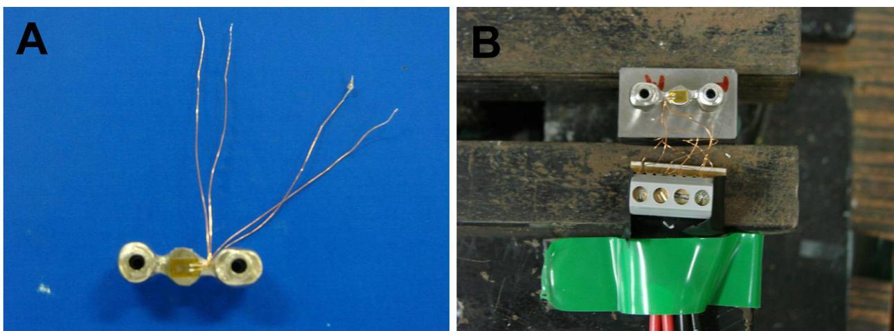
**Fig. 2.** Experimental setup with extensometers. **(A)** Extensometers glued to the upper and lower part of the pontic. **(B)** Extensometers wired to record the output signal during the tests.
