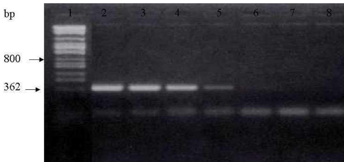
Figure 2. Electrophoresis in 1.2% agarose gel stained with ethidium bromide, showing the results of the sensitivity assay for CFU/mL in sewage samples contaminated with Shigella dysenteriae after enrichment culture. (1) \lambda ( Eco RI/ Hind III/ Cla I); (2) 10 5 CFU/mL; (3) 10 4 CFU/mL; (4) 10 3 CFU/mL; (5) 10 2 CFU/mL; (6) 10 1 CFU/mL; (7) 10 0 CFU/mL; (8) negative control.
