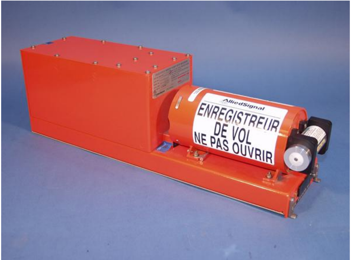
Figura 2.1.6: Flight Data Recorder (FDR) Atual Fonte: National Transportation Safety Board (2004).
