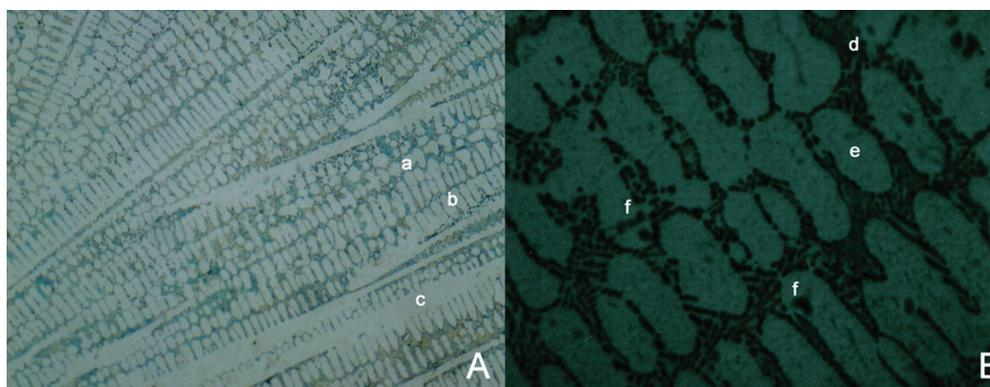
**Fig. 2.** Microstructure of Ni-Cr-Mo-Ti alloy surface at 50x (A) and 250x (B) magnification. (A) gamma ( $\gamma$ ) primary phase and gamma-prime ( $\gamma'$ ) second phase (light region). (B) d) interdendritic regions; e) gamma ( $\gamma$ ) grains; f) Precipitates (Mo or Ti) in the dendritic cores.
