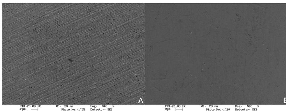
**Fig. 1.** (A) SEM of Ti-6Al-4V surface at 500x magnification: defects of machining results: small pits, irregular scratches. (B) SEM of Ni-Cr-Mo-Ti alloy surface at 500x magnification. Equally smooth surface structure and texture, minor irregularities result of machining and light scratches.
