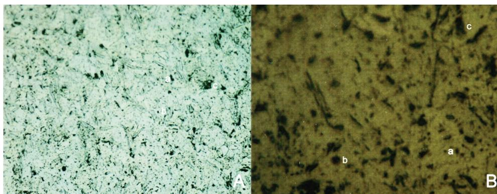
**Fig. 3.** Microstructure of Ti-6Al-4V surface at 50x (A) and 250x (B) magnification. (A) binary (alpha+beta) structure was revealed. a)  $\alpha$  grains; b) precipitates; c)  $\beta$  grains.
