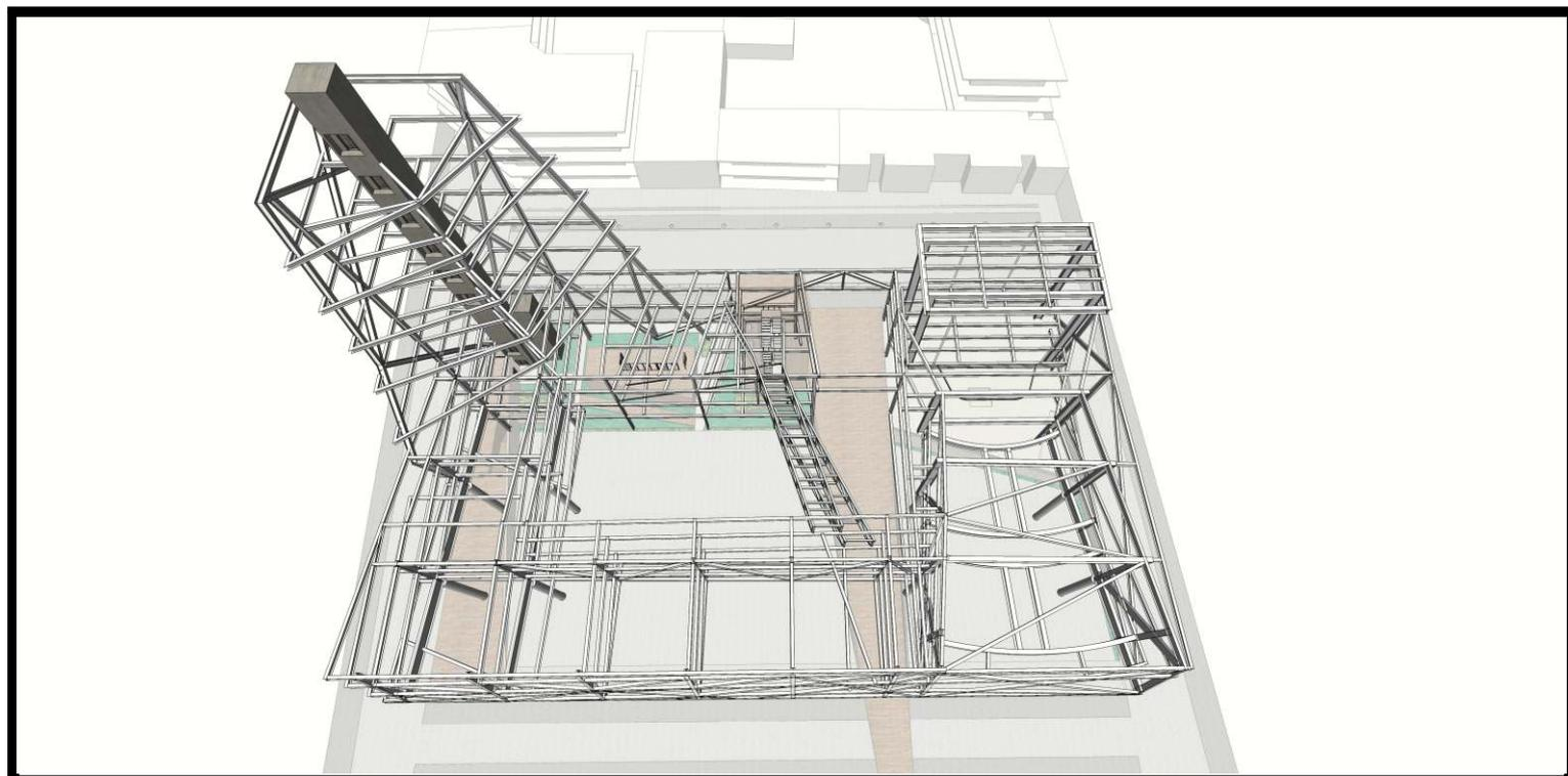
ESQUEMA ESTRUTURAL BÁSICO (VIGAS E PILARES) - SEM ESCALA
