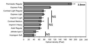
**Fig. 2.** Comparison of optical density mean values of the tested impression materials with 1.0mm-, 1.5mm-, and 3.5mm-thickness. Vertical bars connect means that are not statistically different (*P*>0.05).
