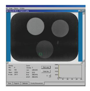
Fig. 1. Evaluation of the optical density of one 1.0mm-thick sample in a 20x20 pixels area using the Digora system.
