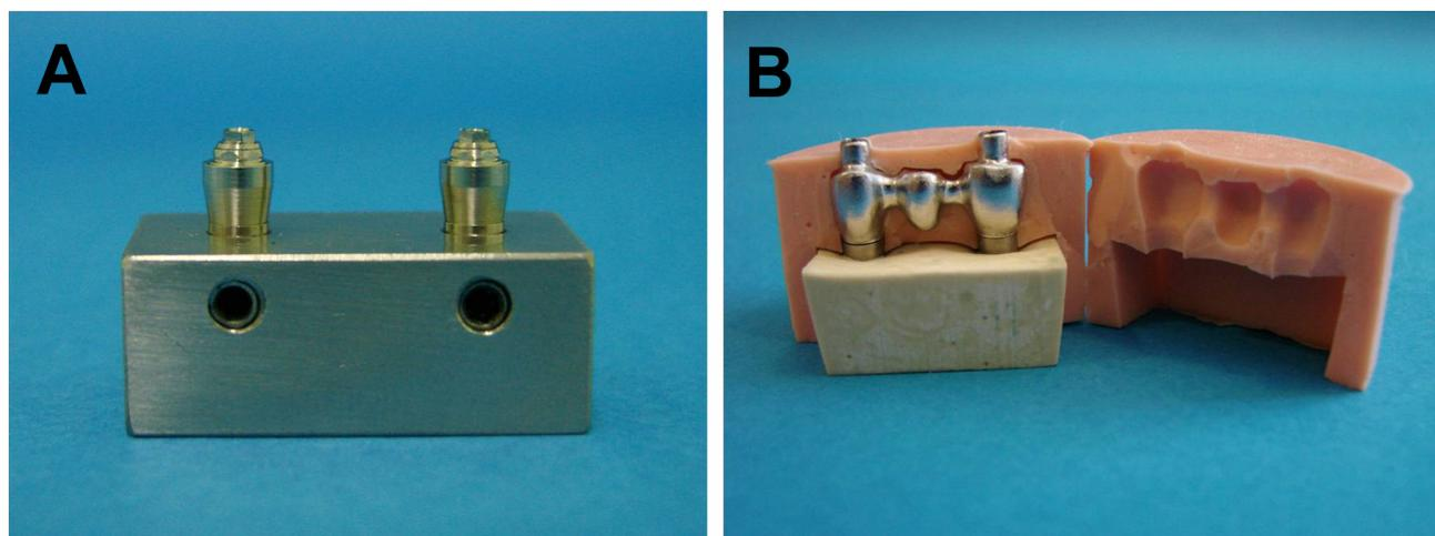
**Fig. 1.** Fabrication of the test specimens. **(A)** Implants installed on the metal base. **(B)** Silicon index utilized to standardize the framework waxing-up.
