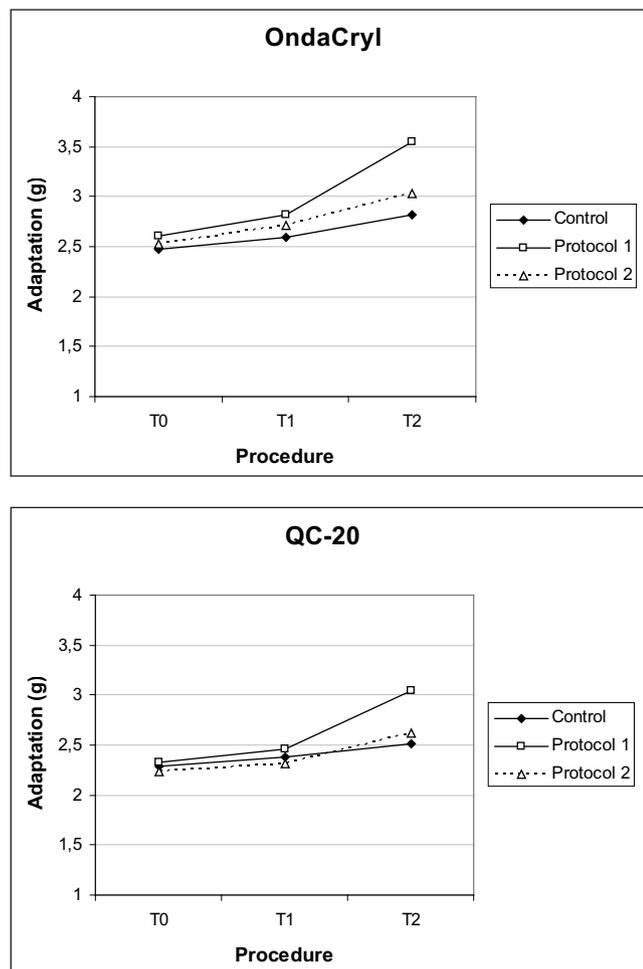
**Fig.2.** Baseplate adaptation mean values (in grams) of OndaCryl and QC-20 resins according to disinfection treatment groups and number of disinfection procedures. Control and Protocol 2 (345 W/6 min) groups showed similar behavior. Significant poorer adaptation ( $P < 0.05$ ) was measured after two microwave disinfection procedures with Protocol 1 (690 W/6 min).
