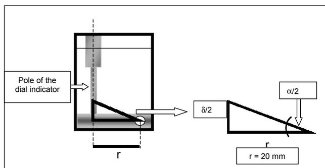
Figure 1 – Graphic representation of the device used to measure rotational freedom, where [r] = bar radius, [α] = angle formed during the bar displacement, and [δ] = displacement of the bar, which moves the pole of the dial indicator. The circle indicates the place of fixation of the implant/abutment or implant/analog.
