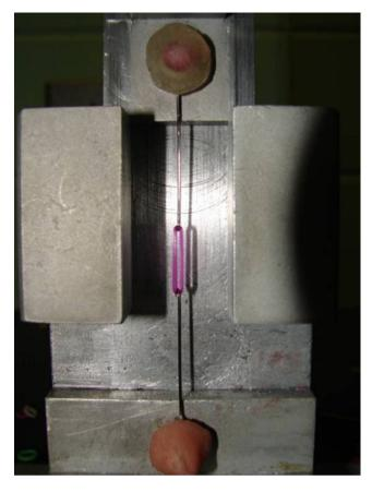
Fig. 1. Device for traction of plastic bands attached to the trial universal machine.
